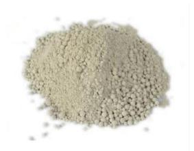
Alumina hollow ball castable is a high temperature refractory and thermal insulation material made of alumina hollow ball. Its service temperature is 1600-1700 °C, its load softening temperature is high, its strength is large, and its thermal insulation performance is good. It is often used for the lining of carbon black reaction furnace and high temperature furnace.
